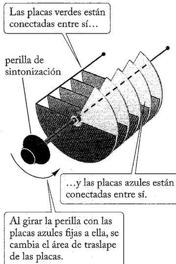
**FIGURA 26.5** Un capacitor variable.
