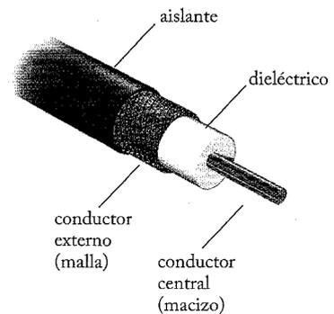
**FIGURA 26.19** Cable coaxial.
